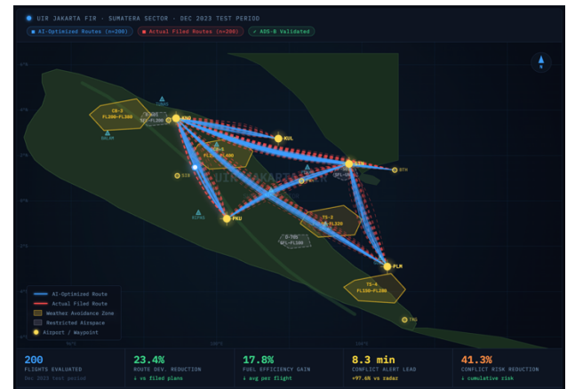
Fig. 2. Comparison of AI-optimized routes (blue) versus actual filed routes (red) over Sumatera airspace, with GIS overlay of weather avoidance zones (yellow polygons) and restricted airspace (grey). December 2023 test period sample of 200 flights.
